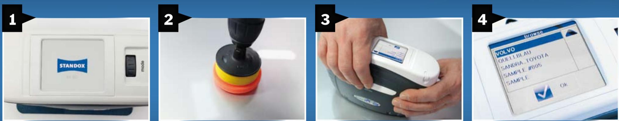
In order to deliver flawless results, the Genius device with the help of its associated blue and white standards should be calibrated regularly. The standard must be kept clean at all times. Tip: for cleaning use warm water and a soft cloth. Do not use solvents or polish.
