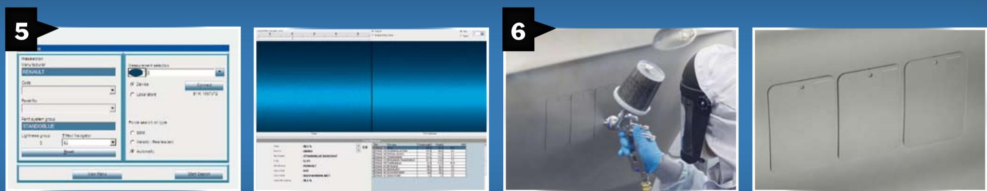
The Standowin software shows all hits as a list - based on the values and color icons, (for color and effect accuracy) the optimum formula is selected quickly and easily.
