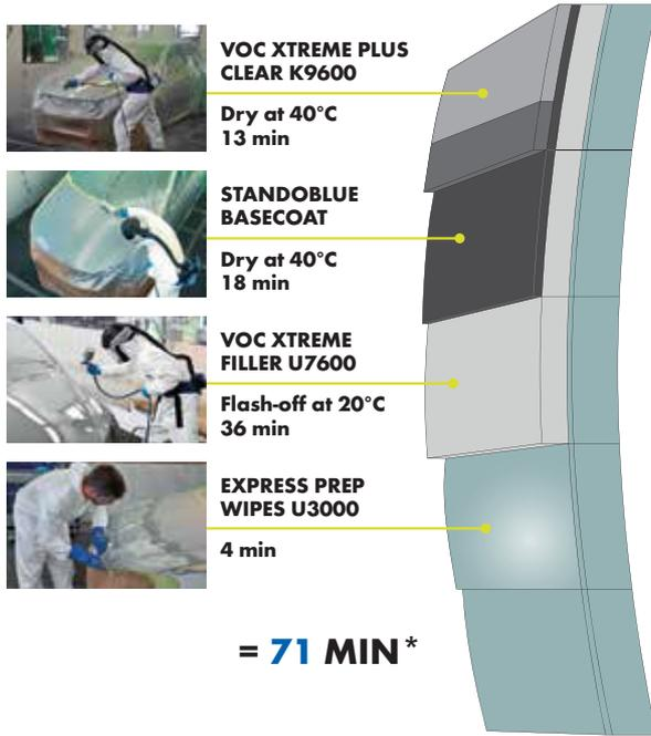
\*71 minutes repair time is based on a standard repair of 3 panels, including bare metal repair to bonnet needing primer filler application. Includes application, flash-off and drying times.
