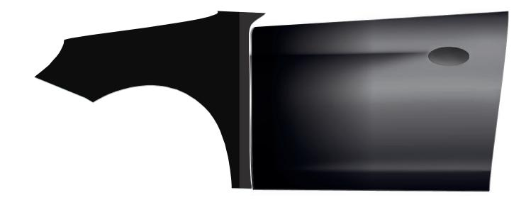
• Apply Effect Colour in 3-5 even coats to the part to be painted and the repair part. Allow to flash off.
