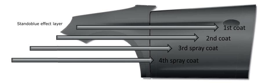
Before applying the clearcoat, check the application of the effect layer with a daylight lamp, making sure that the groundcoat is completely covered in the transition area.
