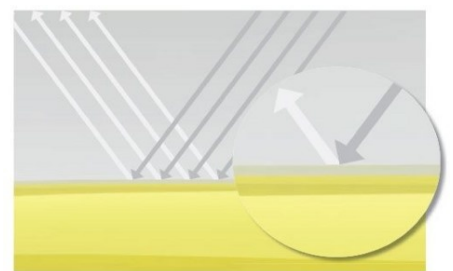
Light reflection on a glossy clearcoat (simplified illustration, as effect pigments also have a scattering effect, although only in the basecoat paint).
