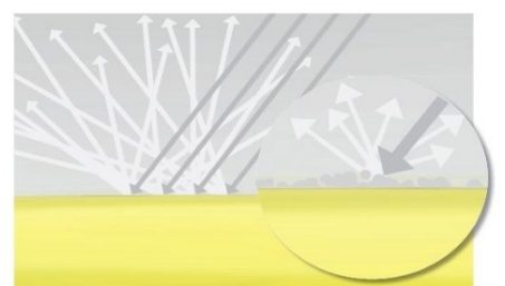
Light reflection on a matted clearcoat (matting agents contain ball-shaped particles that have a strong scattering effect). Viewed at an angle of
