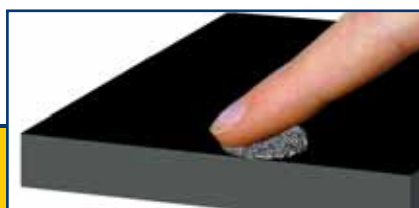
Rust caused by impurity: Rust can even be caused by a fingerprint on bare sheet metal.
