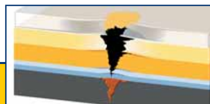
The consequence: Rust starts to form under the paint coat.
