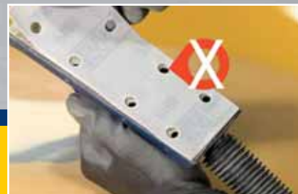
WRONG Wrong abrasive or the abrasive is not positioned squarely on the sanding block.
