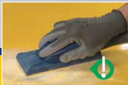
RIGHT The flat sanding area distributes the pressure perfectly, hollows and holes are avoided, the abrasive is fully used.
