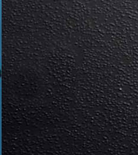
above: Pinholes are caused when the paint is applied too soon.
