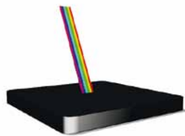
Light falls on a black surface. The complete colour spectrum is absorbed.
