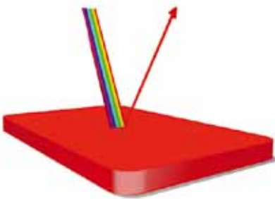
Light falls on a red surface. The component of the colour spectrum is reflected, the remaining light is absorbed.
